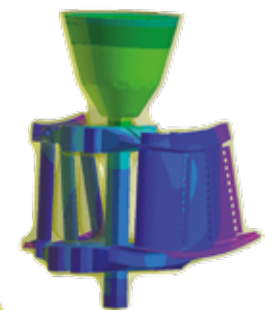
NGV Blade with Realistic Shell Modelling
